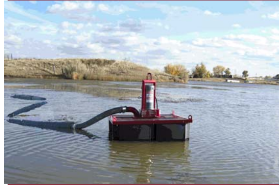
SRS Crisafulli Floating Pump with Discharge Tubing
