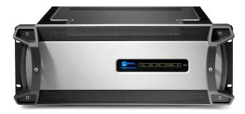
PowerStation is what we Axians refer to as an "integrated console engine", an all-in-one titan that makes it easier than ever to install Axia studios with Element consoles. Inside that ruggedly handsome case you'll find a super-powered DSP mixing engine, husky power supply sourced from telecom gear designed for harsh environments, plenty of built-in digital, analog and mic I/O, plus EQ, voice processing — and even a custom, built-for-broadcast Ethernet switch with Gigabit connectivity.
