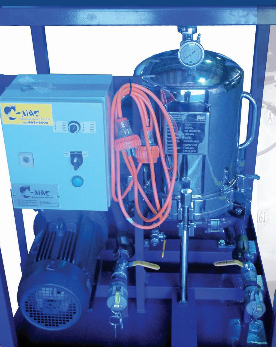
Small mobile transfer filter pump has been developed to filter 4,000 litres per hour of contaminated oil with a capability of filtering down to 5 microns of particle size.
