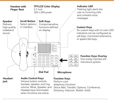
**Note:** You can connect a supported headset into the 265 IP Phone by plugging the headset into the headset jack at the left corner of the phone chassis. Contact your system administrator for details.
