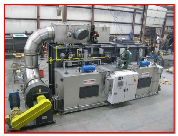
*Hot Air Recirculation* – mixes clean hot oxidizer exhaust with cold wet inlet gas to insure re-vaporization of condensing water vapor prior to entering the EvenFlow Manifolds.
