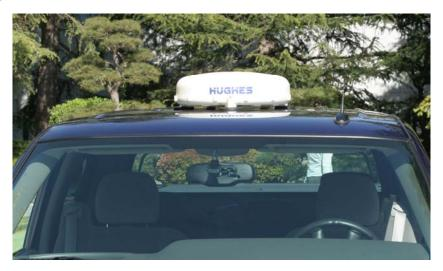
The Hughes 9250 Broadband Satellite IP Terminal and WLAN Access Point is your gateway to mobile communications. It allows you to send and receive IP packet data via Ethernet and WLAN interfaces over the Inmarsat BGAN satellite network in a land-vehicular application. In parallel with the packet data services, the same terminal supports a circuit switched voice call or a 64kbps ISDN data call.
