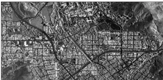
ORI – Pixel Resolution: 1.25m, Horizontal Accuracy: 4m CE90%.
