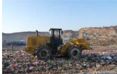
b) field compaction test
