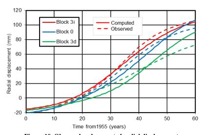
Figure 10. Observed and computed radial displacements.
