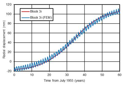
Figure 8. Adjustment of movements in block 3i.
