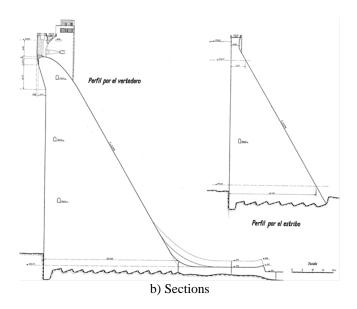
Figure 5. Drawings of the arch gravity dam.
