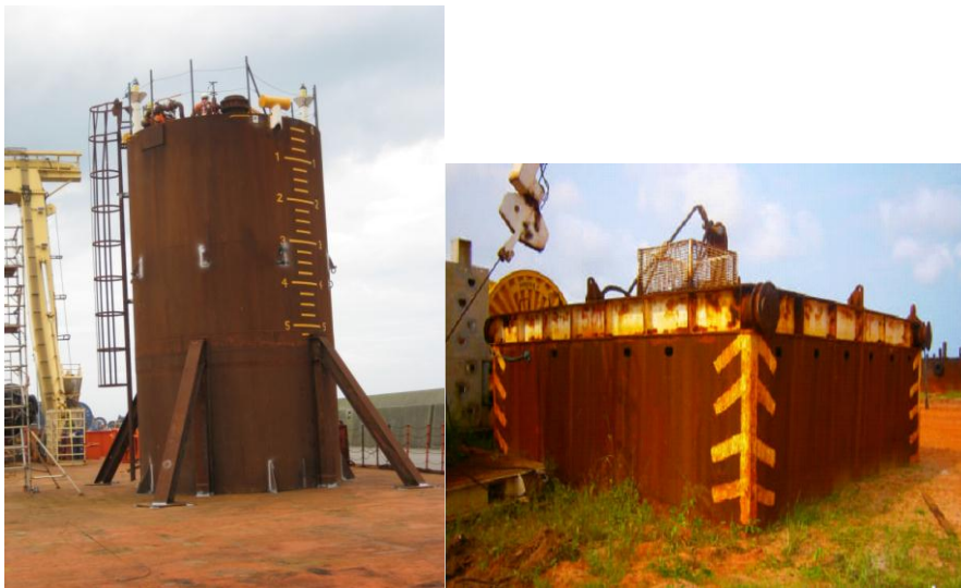
Figure 9. Suction pile (left) and gravity base (right) anchoring mitigations
