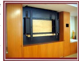
The RPV RPPM-Flex Mount is CNC laser cut from precision formed 3/16” black powdercoat welded steel. This heavy duty robust steel fabricated mount can extend out from the wall up to 31.5”, allowing an installer, service person, or end user to physically get behind the mount for cable connecting and trouble shooting. Additionally, the mount articulates left/right to enhance the viewing experience and for ease of installation/service.
