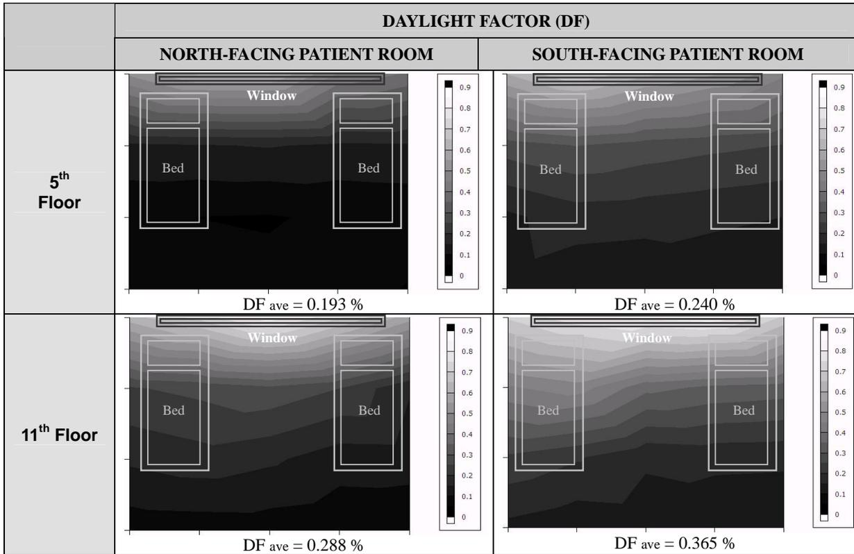
As depicted in Fig.4, the Daylight Factor is lower in the lower floors and higher in the top floors (11<sup>th</sup> floor). This occurs because the surrounding tall buildings block the view to the sun and sky. Thus, this building can generally only have daylight after 9:00 AM during the fall season. The daylight in the southeast-facing patient rooms is more introduced than in the northwest-facing patient rooms.
