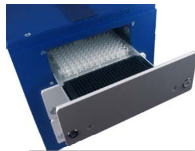
All MéCour thermal units are connected to circulating baths for total uniform and stable temperature.
