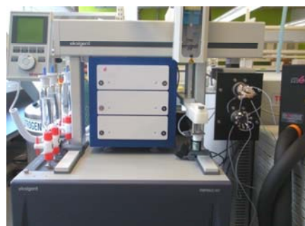
Same platform integrated with MéCour temperature control solutions for sample storage, valve and column temperature control
