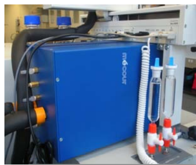
All MéCour thermal units are connected to circulating baths for total uniform and stable temperature.
