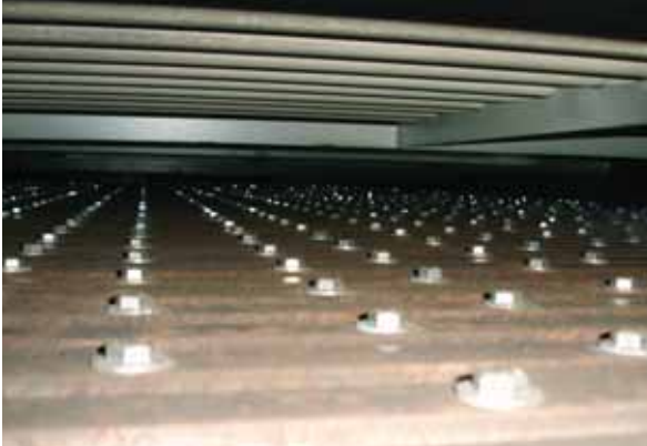
Gas distribution plate designs to enhance material flow and minimize back-sieving
