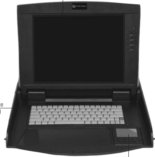
Touch pad buttons operate in dual mode, use buttons or touch pad for mouse click.
