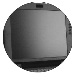
15" TFT color display supports screen resolutions up to 1024 x 768
