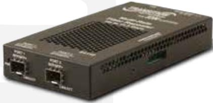
The S4110-4848 is a 10Gbps protocol independent media converter with two pluggable SFP+ ports. Each port can support data rates from 1Gbps up to 11.5Gbps allowing network designers to customize the S4110 with a pair of SFP modules from Transition Networks' wide SFP product offering, to meet their network requirements. The S4110-4848 can be used as an any-rate to same-rate fiber mode converter, as well as a WDM transponder.
