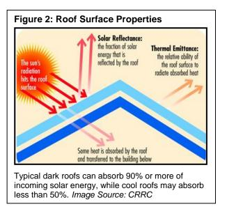
increase the heat flow into the building, causing the air conditioning system to work harder and use more energy in summertime. In contrast, light-colored roofs absorb less than 50% of the solar energy, reducing the roof temperature and decreasing air conditioning energy use.
