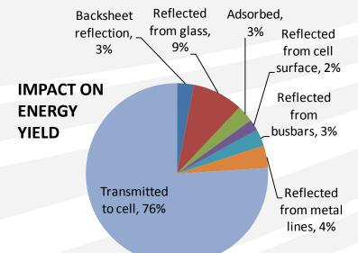
Assumptions: Incident sunlight, No ARC on glass, 4mm low Fe glass, 0.5mm EVA encapsulant, SiN ARC on textured cells, 7.5% of cell area is metallization, 93% cell packing factor in module. Excludes frame and edges. Energy yield is calculated for 33° on 07/01/2010 at 42° latitude. **Note:** Actual transmission to cell = 65% to >90% depending upon technology, architecture and orientation
