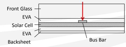
Local Roughening with Laser to Introduce a Scattering Surface
