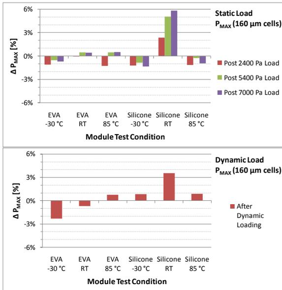
Figure 3. Change in maximum power output of test modules made with 160  $\mu$ m cells after static (top) and dynamic (bottom) loading. The percent change is relative to the unloaded module.
