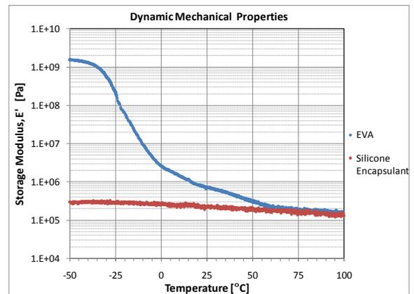
**Figure 7.** Storage modulus of silicone and EVA encapsulant measured using DMA in tension mode.
