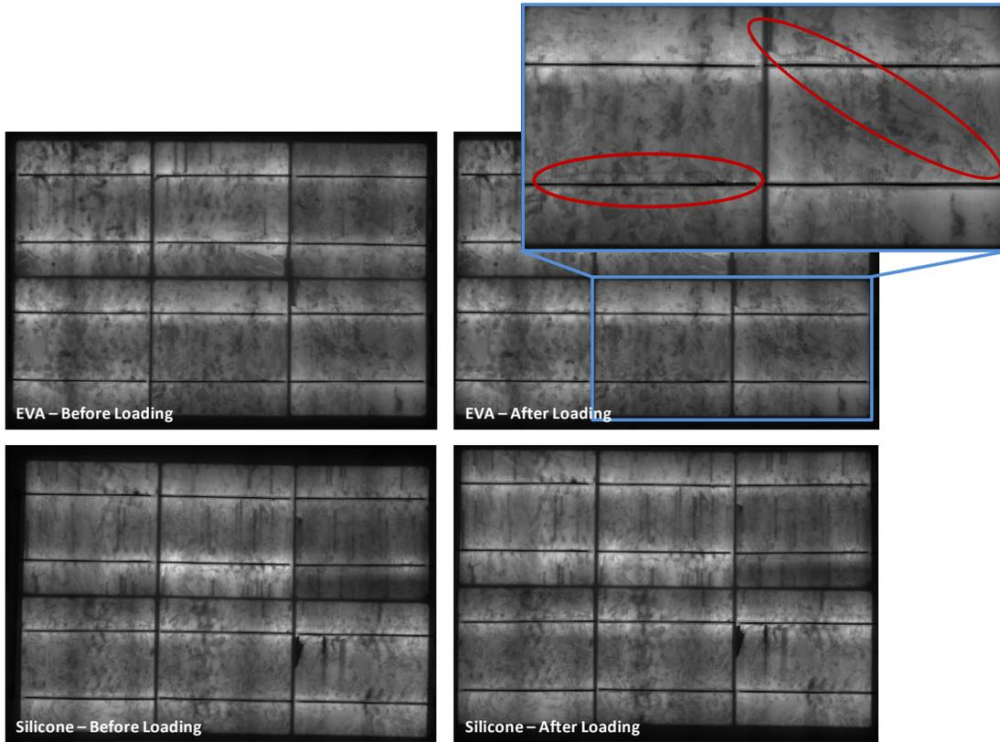
Figure 2. Electroluminescence images of modules after static loading to 5,400 Pa for 1 hour at ambient temperature. Cracks were observed to form in the module with EVA encapsulant, whereas no new cracks were seen in the module with silicone encapsulant.
