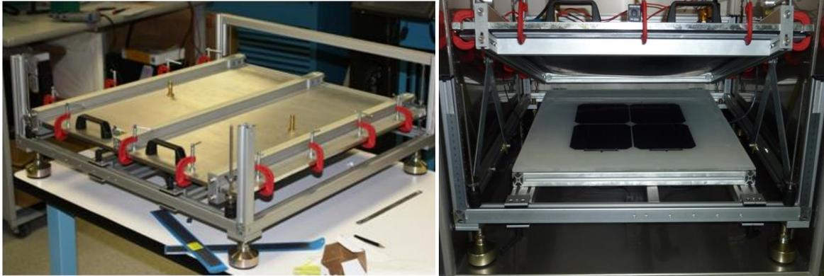
**Figure 1. Custom built mechanical test stand for load testing of test PV modules inside a climate chamber. The image on the right shows a test module inside the stand with the rubber bladder seen above, attached to the top plate.**
