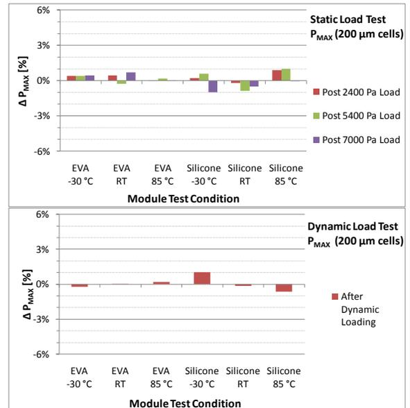
Figure 4. Change in maximum power output of test modules made with 200  $\mu$ m cells after static (top) and dynamic (bottom) loading. The percent change is relative to the unloaded module.
