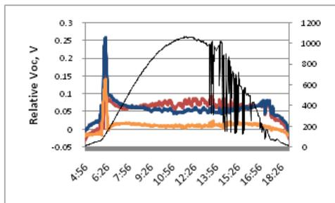
**Figure 10:** Difference in  $V_{oc}$  between structured glass and reference module: Grooves (red), pyramids (blue), and lightly textured (orange). Irradiance (black,  $W/m^2$ ) is also shown. Sharp peaks near 6:00 AM are due to discontinuous measurements recorded by the DAQ system. Data is from May 22, 2010.
