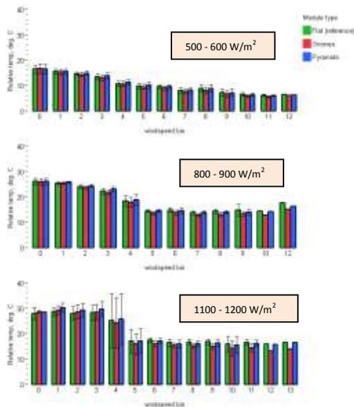
**Figure 13:** Module temperatures, relative to ambient temperature, vs. wind speed bin (m/s), for three levels of irradiance.
