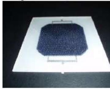
**Figure 4: Pyramid glass one cell module**
