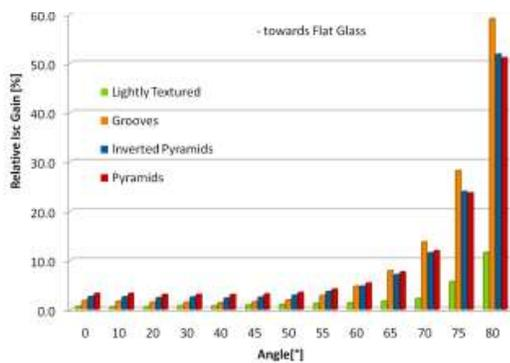
**Figure 7:** Effect of textured glass on  $I_{sc}$  as a function of angle of incidence
