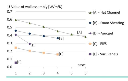
high-end materials, as aerogel and VIP, can be seen as an outlook: as soon as they are available on economically acceptable scale, they are solutions if the amount of space is limited or installation of exterior insulation is prohibited
