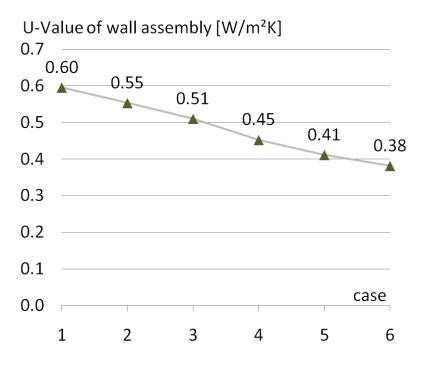
example A) metal spacer, variation of conductivity of insulation material in the cavities
