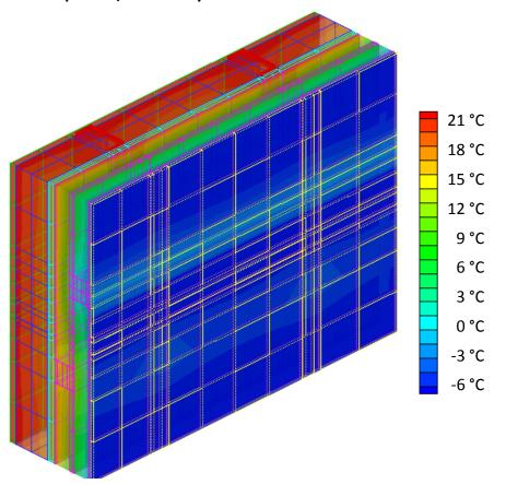
By using materials with very high thermal resistivity the influence of the metal studs is nearly insignificant.
