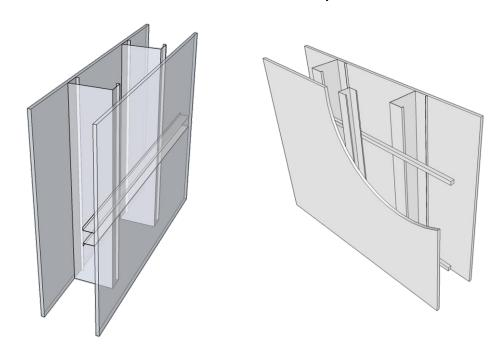
example A) metal spacer, variation of conductivity of insulation material in the cavities
