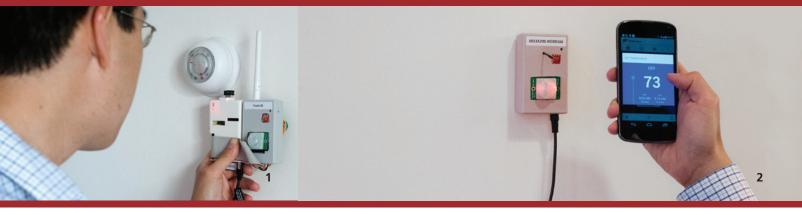
1 Controlling a residential thermostat using a sensor hub and remote wireless node.
