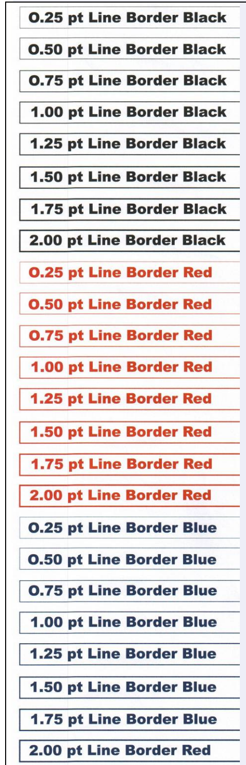
This cropped image of a BERTL test pattern examines the reproduction capability of fine lines in multiple colors. The Océ ColorWave 600 printer has no problem in reproducing fine lines.
