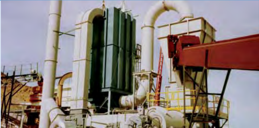
Complete Fluid Bed Dryer System Used in the Mining Industry
