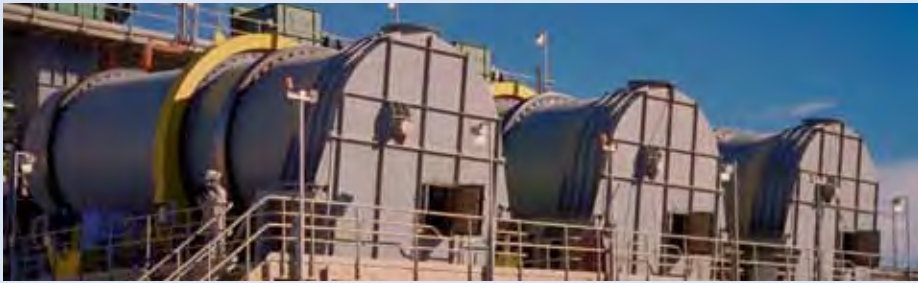
Rotary Agglomerator/Granulators Used to Process Copper
