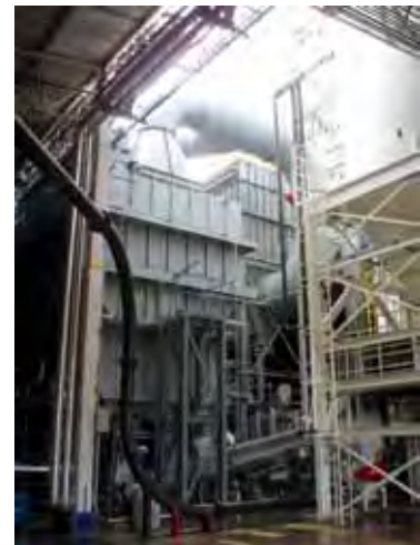
Fluid Bed Dryer Used for Spent Grain
