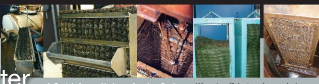
A Crutch for an Underperforming Coalescer When insufficient coalescer design was recognized, especially in the below ground cylindrical market, manufacturers had to come up with a way to promise stated removal values. These "polishing" packs readily plug at their entrance points, and actually serve as a flow obstruction within the treatment.
