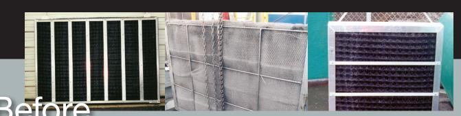
Secondary Treatment These packs of tightly bound plastic or steel fibers are used as a secondary coalescer designed to be a last catch basin for any small oil droplets not removed during the primary treatment.
