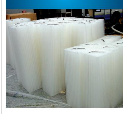
the media from a tank. The idea is to tightly pack the entire volume of the tank with these bundles, and remove them for cleaning when necessary.
