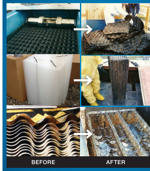
A Clogged Coalescer Leads to Decreased Oil Removal
