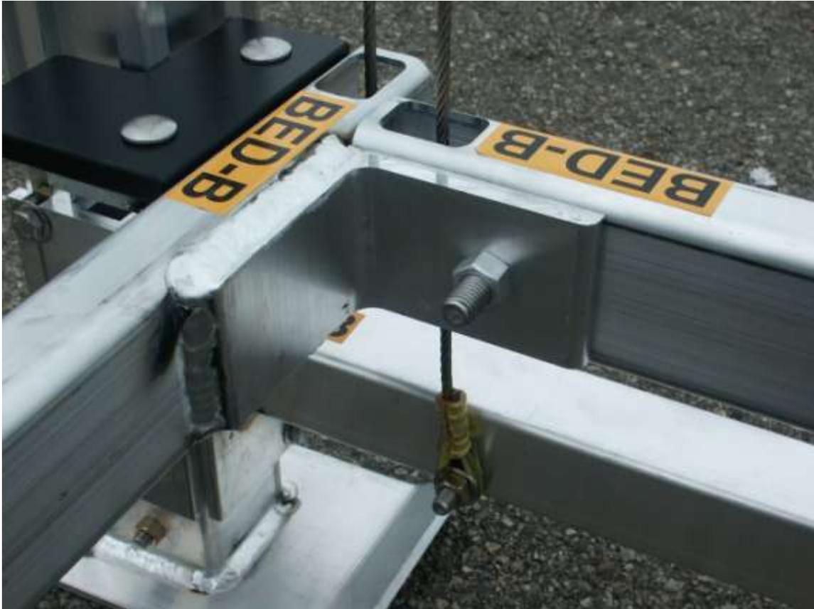
Without removing the 1/2-13 SS screw, remove the aluminum 1/2-13 nut from Front Beam ('Bed B – Bed C' beam), again DO NOT REMOVE THE 1/2" SCREW. Slide the 1/2" screw onto the welded angle of the Side Beam ('Bed A – Bed B'). Finger tighten the aluminum screw. Repeat this for the remaining 3 corners. Tighten all screws. Double check pulley clearance. Note: pulley may seem to drag due to the cable wrap, pull the cable free from the pulley and recheck.
