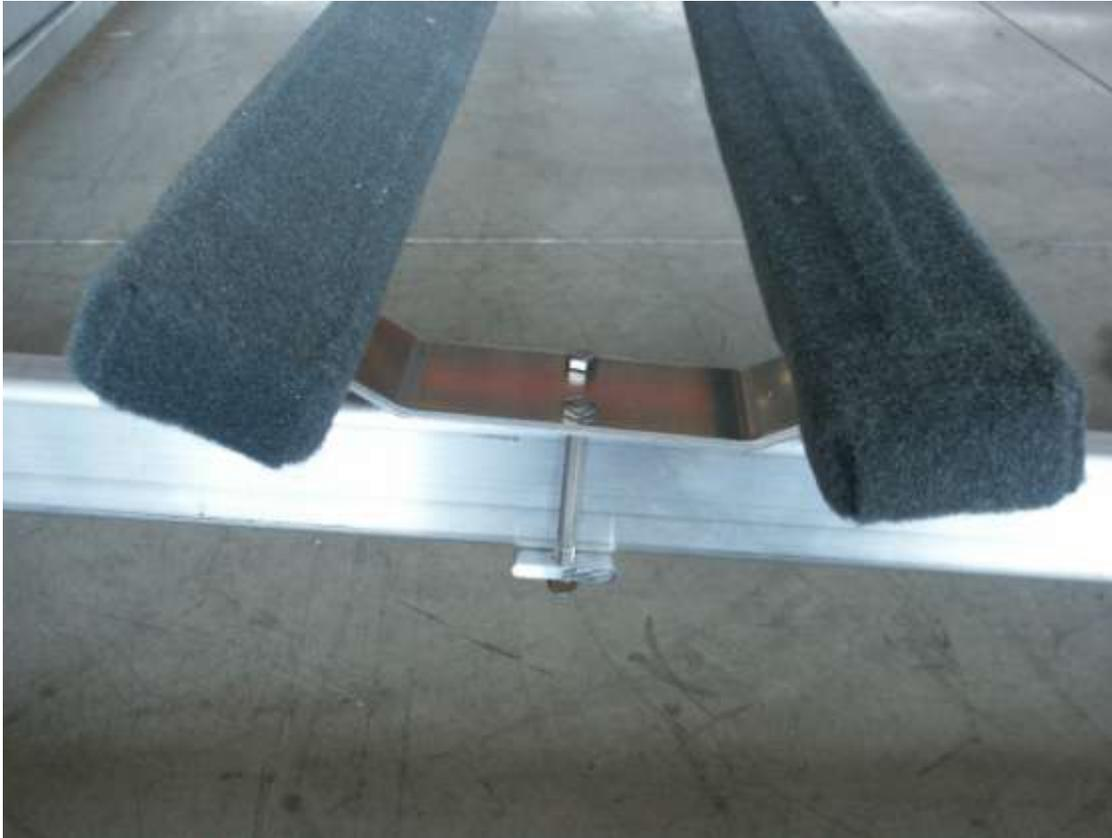
Turn bunks upside down and attach the aluminum Bunk Support using the 5/16 x 1.5" lag screw to the bunks. Once both bunks are attached to the 2 brackets, attach the assembly to the Bed Beam using the 3/8" x 4" hex screws, Bracket Backer Plates and brass hex nuts as shown. Adjust width to match hull width.
