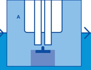
It is important to remember that maximum results can only be achieved through central alignment of the female channel to the creasing matrix.
