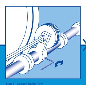
Using a 4mm Hexagon key loosen the existing Muller arm (the thread will be found on the underside of the arm) See diagram above.
