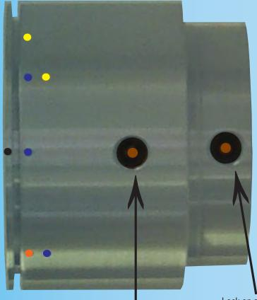
Loosen this allen screw to rotate collar for channel width adjustment Lock on shaft using this allen screw
