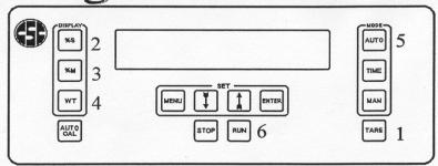
1) Turn power ON. Switch is located at the left rear of the instrument. (This switch may be left in the ON position at all times to eliminate the need for warmup.) Allow the CSC Digital Moisture Balance to warm up for 20 minutes before starting operation. \*NOTE if the instrument is not allowed to warm up for this time, the results of the first test may not be accurate.
