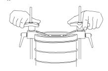
down simultaneously to ensure the clamping plate is square. Continue until the handwheels are tight against the internal stop. Hand tightness must be exerted so that the assembly does not loosen during vibration.
