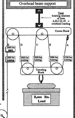
Next we can determine the lead line tension at the winch when the load is being hoisted by counting the number of line sections from dead end to winch end, in this case line sections A through H = 8.
