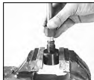
Step 4 — Bottom tube end firmly on internal shoulder of Ferulset Tool (or fitting body).
