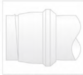
Fig. T50 — Ferrule cocked on tube
