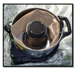
STEP 7: Connect the new collection bag. Make certain that a good seal has been created between the bag and the canister intake.
