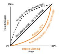
The flow rate of a conventional two-way valve depends upon both the degree of opening and the pressure. For example: a valve that is 50% open and supplies 5 GPM at 4 PSI, will at 36 PSI, supply 15.0 GPM at the same opening.
