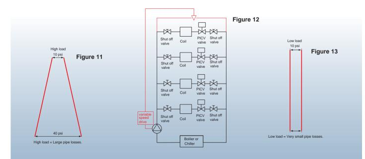
Example: set point for pressure control = 10 psi. Pressure drop at full load is 30 psi between supply and return. This means that the pressure at the first valve is 30+10 = 40 psi at full load. At low loads on the other hand, the pressure approaches 10 psi, as the pipe losses goes down by the square. At full load (40 psi) we will have problem with a poor valve authority for the first valves, and at low loads (10 psi) we can not supply the full flow.
