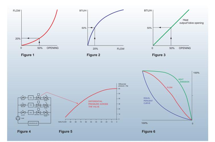
The PICCV valves are used as a replacement for conventional two-way control valves, but offer a very important new feature. It will regulate the flow rate regardless of the differential pressure. In other words, it is a true flow controller.
