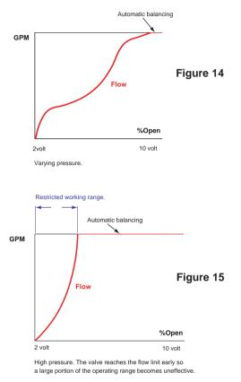
Figure XXX shows the operation of a combination valve as well as the PICCV. As you can see, the limiting valve acts as a conventional control valve (within its differential pressure limit of2-14 PSI) and then resumes the action of a conventional control valve with higher differential pressures.
