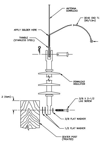
The Symmetrical "T" Antenna is recommended if sufficient land is available. This antenna requires a plot of ground approximately 150 feet by 350 feet. The calculated range with the "T" Antenna and a 25 watt transmitter is 80 to 100 miles except over low conductivity ground. The standard "T" is electrically very similar to a 1000 pF capacitor in series with a small resistor.
