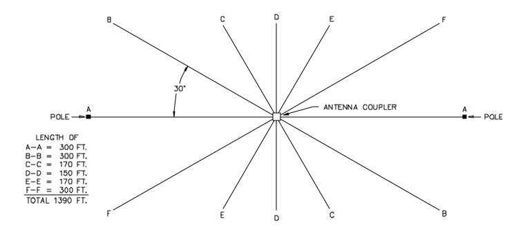
The counterpoise system should be laid out as shown above. The dimensions above are not critical in normal soil and may be altered slightly is necessary. 1500 feet of #10 bare solid copper wire is supplied, which is more than sufficient for the standard counterpoise system.
