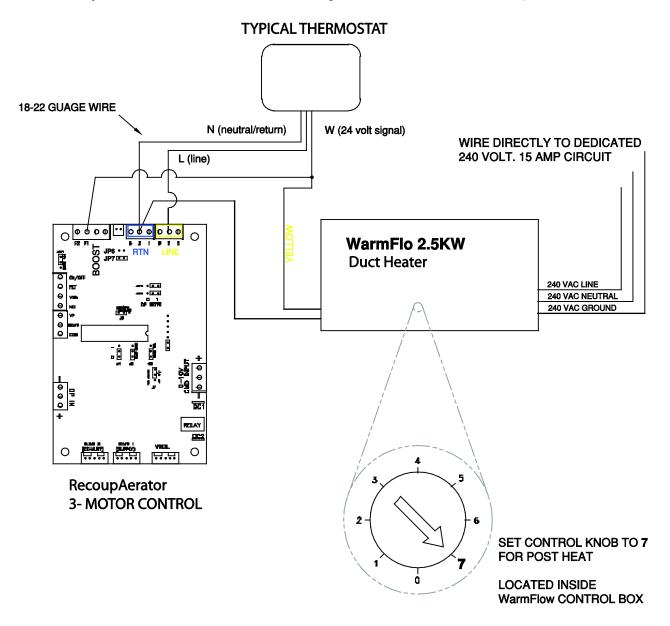
Note: If an external 24VAC source is used remove both jumpers 6 & 7. For example, removing both jumpers 6 & 7 allows control by a furnace 24VAC source while safely isolating the *RecoupAerator*'s 24VAC system.
