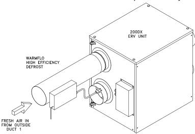
**3** Set the Output Temperature to position "2". The Temperature Setting knob is inside the WarmFlo control box. The *RecoupAerator* is designed to shut off below 10°F, and the WarmFlo Defrost Heat is meant to keep the Fresh Air Inlet at above the *RecoupAerator* frost protection shutoff temperature. The WarmFlo Defrost Preheat ensures the *RecoupAerator* provides a Fresh Air supply below freezing temperatures.
