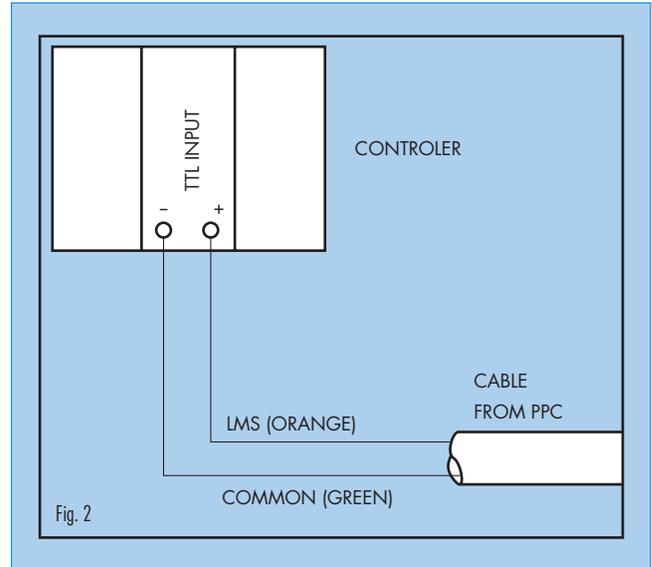
There also is a negative logic version (LMS) available. When the correct pressure is achieved, this option outputs a logic 0. When the PPC is working (fill or exhaust valve is in operation) the output is a logic 1. In either case, the LMS circuit is a sinking type of output. Thus, the PPC supplies the ground to the reading device.
