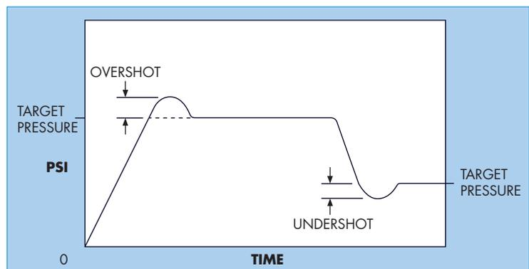
The PPC is based on a closed loop design which combined with MACs fast responding, very repeatable, high flow, balanced 2-way valves, optimizes response and accuracy, practically eliminating overshoot and undershoot.
