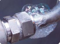
system components demonstrated through the use of a hydrostatic burst test.
