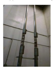
pffels is the most state-of-the art automated coffee roasting facility in the world. From roasting, to blending, to packaging, the coffee is transported through air-tight conveyor tubes with no human hands ever touching the coffee! Also see the conveyor tubes in the photo on the right.
