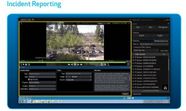
When monitoring an incident, the user interface can play a role in how quickly information is retrieved. Users can leverage the Tagging feature in the VideoXpert Ops Center to tag cameras to quickly identify cameras linked to the iTrak system. Users can select from alternative UI views to only show an incident when needed.
