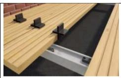
**Step Six:** Choose any of the four spacing options available on the Deck Spacer, Flip the board over and slide it into place. The unfastened end will be held in place by the prior row of decking. Fasten the other end of the Deck Glider to the joist.
