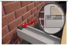
Step One: Start your decking installation by screwing the female end of the Glider Starter Clip onto the Aluminum System Profile. The male end of the Glider Starter Clip is screwed onto your first decking board.
