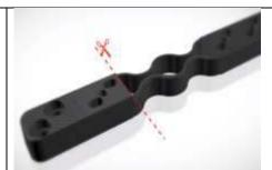
**Step Two**: Cut off the 'fastening end' of a Deck Glider (the one that has two screw holes on the end). This piece will be screwed into bottom of the deck board in the appropriate place to line up with your aluminum joist.
