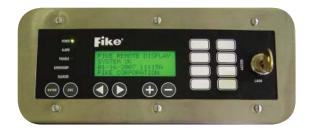
The FRD also includes six buttons (Enter, Escape, ±, left/right arrow) that are used for navigation through events as well as configuration of the device. In addition to the navigation function buttons there are eight programmable buttons that can be configured for things such as reset, silence, acknowledge, drill, or process. This unit includes a key lock access for additional security.
