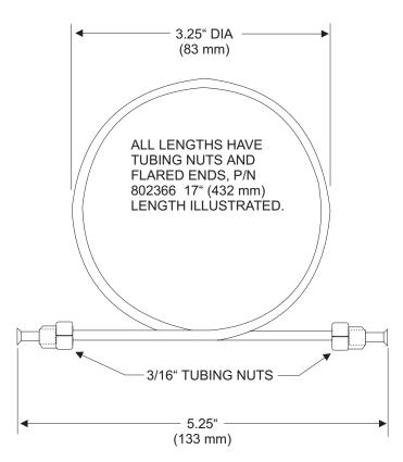
MATERIALS TUBING: COPPER TUBING NUTS: BRASS
