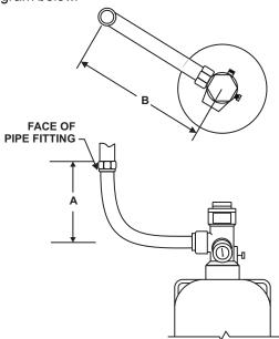
Note: Dimensions A and B must be maintained in order to obtain a smooth radius in flexible loop. Hose may require adapter to connect to system piping.
