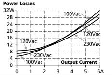
Fig. 9-4 Losses vs. input voltage, 48V, 5A
