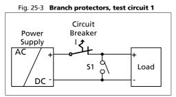
Parameters: Input voltage: 230Vac, load current: 0A
