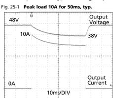
Peak load 10A (resistive) for 50ms Output voltage dips from 48V to <u>38V.</u>
