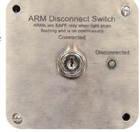
ARMs have discharged their circuitry to a safe level, the ARM disconnect provides a positive feedback indication by changing the LED to a "steady on" state. The ARM disconnect maintains circuit supervision by placing the releasing panel in a trouble condition whenever the key-switch is in the "disconnect" position.
