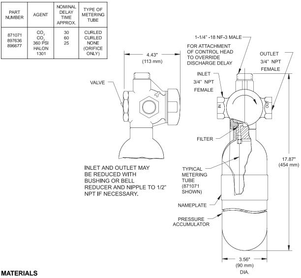
PRESSURE ACCUMULATOR: STEEL **METERING TUBE: STAINLESS STEEL**
