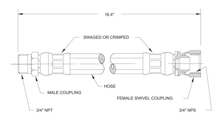
MINIMUM BURST PRESSURE: 11000 PSI (758 BAR) HYDROTEST: 4000 PSI (276 BAR)
